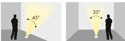
Asymmetrische Linse 45°/35° / Asymmetrical lens 45°/35°
